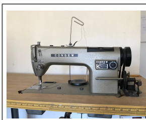
Industrial machine : for strong sewing and high volume sewing Heavy duty Can do thick sewing like leather and vinyl! Used for high output sewing - like sewing done in clothes factories
