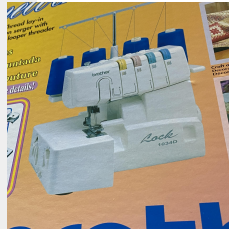
Sergers aka Overlocking Makes the stitches over the ends of fabric It helps keep the fabric from coming apart
